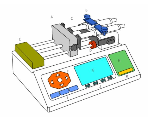
A: Pusher block – locking mechanism varies B: Spring loaded syringe holder C: Withdraw holder D: Safety nut E: Hex allen wrench F: Directional keypad G: LCD Screen H: Numeric keypad I: Stop, Start, Pause buttons J: F1, F2, F3, F4 [Fast forward, Forward, Reverse, Fast Reverse]
