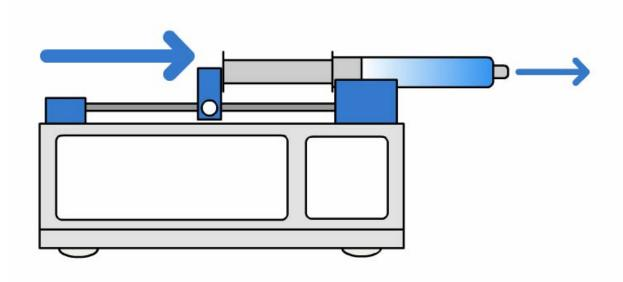
When withdrawing the operation is the same with only the motor reversing direction.
