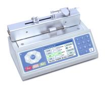
Nanojet is a remotely controlled syringe pump designed for neuroscience use and handling radioactive and highly volatile materials.
