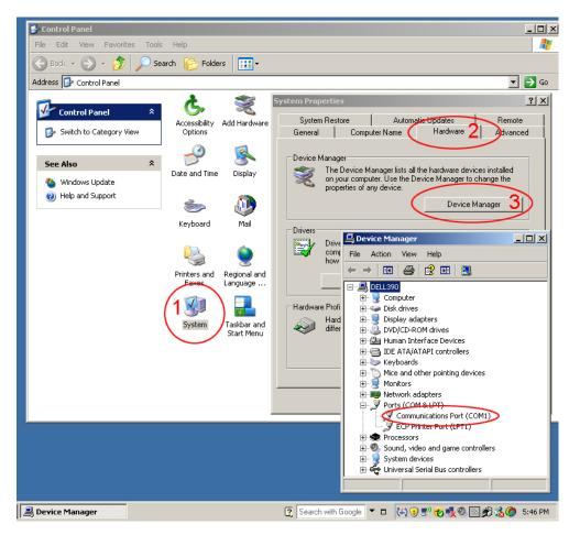
Before interfacing with a PC, make sure a RS232 port exists on your PC. RS232 ports will be in parentheses and named "COM1-100" like the one above named COM1
