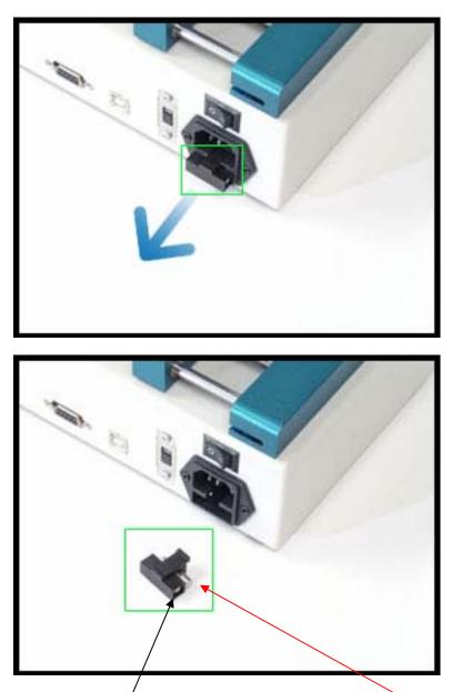
There are 2 fuses in the fuse holder. The exposed fuse in the back is the fuse that is being currently used. In the event of a power surge this fuse will be the broken fuse.
