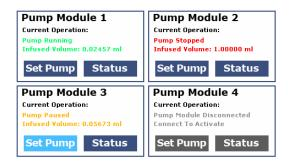
**A)** If the parameter is out of bounds, the pump will show an "effective range" screen for the max and min values at the center of the page. Pump will display "pump running-infusion mode" or "pump running-withdraw mode," based upon the function entered in module "set pump" screen. Once pump has completed running, screen will display, "Pump run finish."
