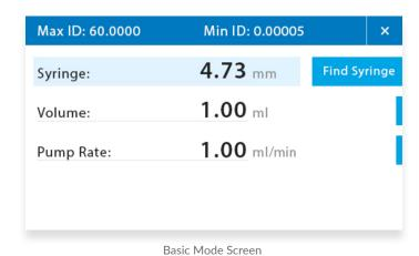
**Basic Mode** (or Single-Step Mode) is used for applications that do not require advanced automation, variable volume and rate settings, step looping, or ramping rates.
