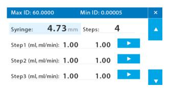
In **Multi-Step Mode**, the left side of the screen shows a list of selectable items. The first (topmost) item in this list is **Setup**. Tapping Setup will take users to the **Multi-Step Method Setup screen**, where the syringe inner diameter (ID), total number of steps, number of loops, and flow-rate units can be set.
