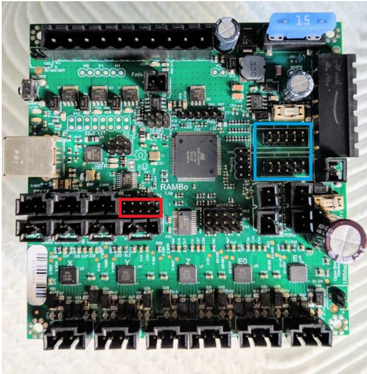
Figure A1: RAMBO 1.4 motherboard. Serial pins highlighted in red, extension pins highlighted in blue.
