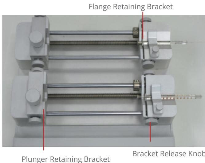
The Fusion 4000-X is capable of both infusion and withdrawal with two independently controlled pumps. The Fusion 4000-X uses adjustable retaining brackets on the pusher block and the syringe holder block, that keep each individual syringe channel in place during infusion and withdrawal.
