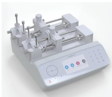
The Fusion 4000-X is a two independently controlled precision syringe pump that allows two syringes to be set up to run simultaneously or independently.
