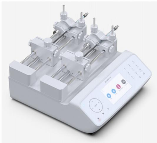
The Fusion 4000 programmable syringe pumps comes with a dual drive system that allows two independent pumping channels to be controlled for simultaneous infusion and withdrawal at same/different flows.
